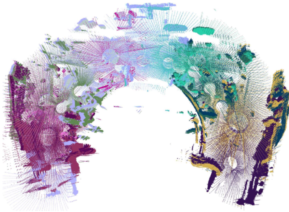
Figure: ICP based indoor map using Mesa and lidar
