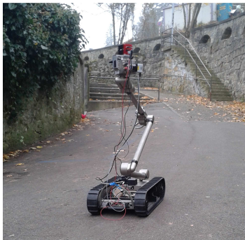
Figure: Robot platform for 2D/3D outdoor perception
